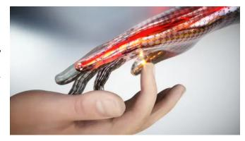
signals into the central nervous system. The materials used in artificial skin mimic the physical traits of skin, incorporating an outer layer of silicone rubber that protects a layer of electronic circuits within. These electronic circuits, which have sensors embedded within them, perform similarly to the body's natural nerves by sending signals that initiate a response to the stimuli.
